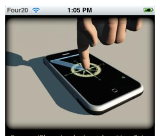
Put your iPhone in a horizontal position. Point your finger at right angles to the center of the compass in the screen. Then turn the iPhone horizontally as the shadow of your finger overlaps the shadow in the screen. Now the "N" on the screen indicates North.
